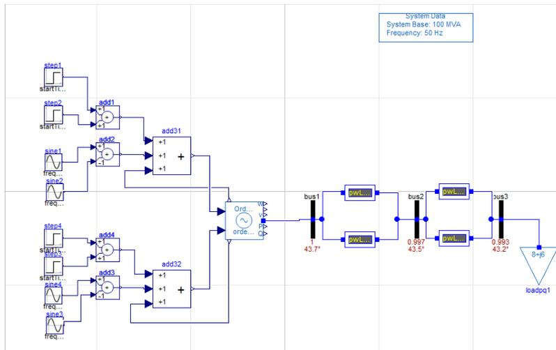
Figure 1: Modelica Implementation of the PQ load test set-up
