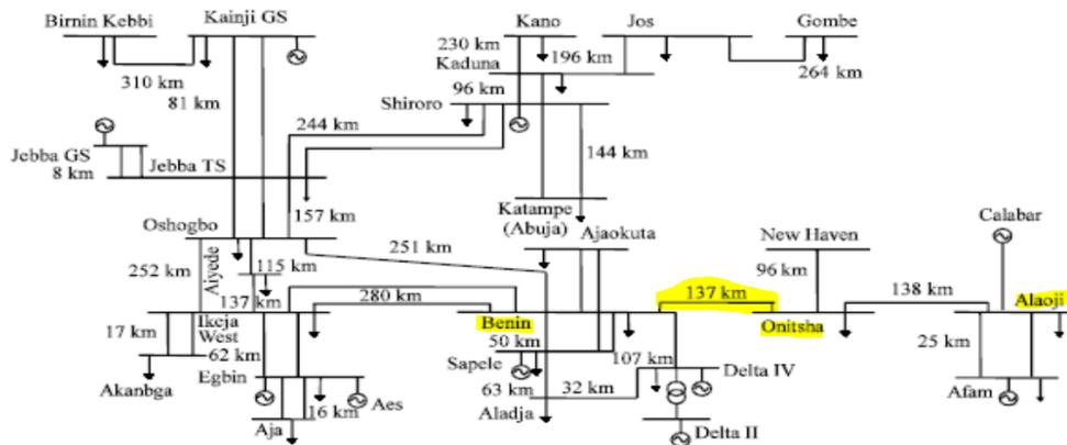
Figure 2: Single line diagram of the Nigeria 330-kV transmission grid
