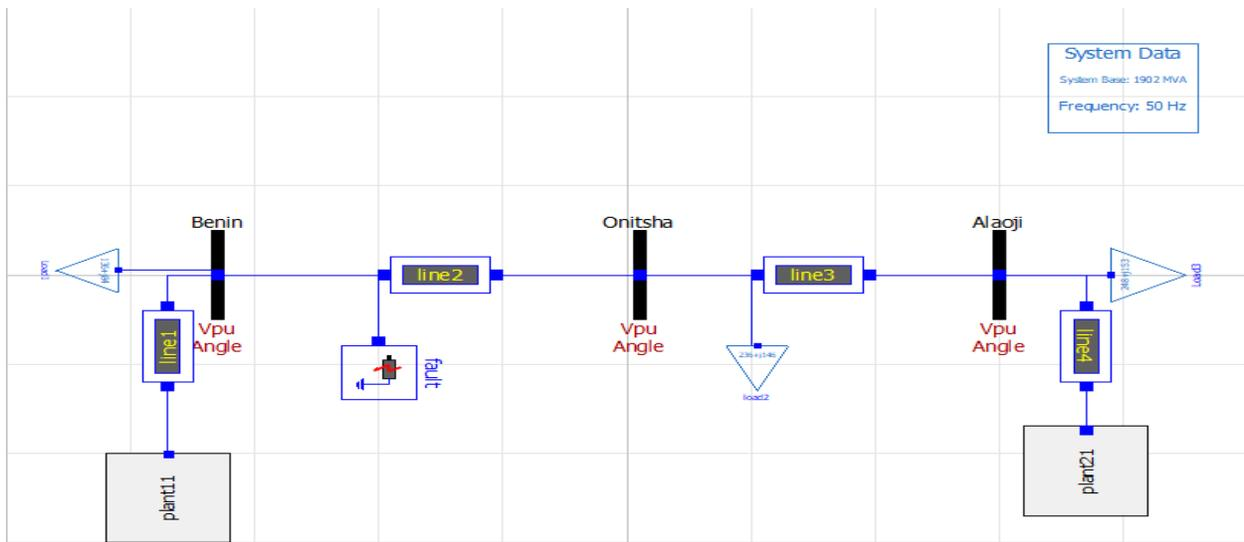
Figure 1: Modelling of Benin, Onitsha and Alaoji lines (330Kv) using Modelica and the OpenIPSL
