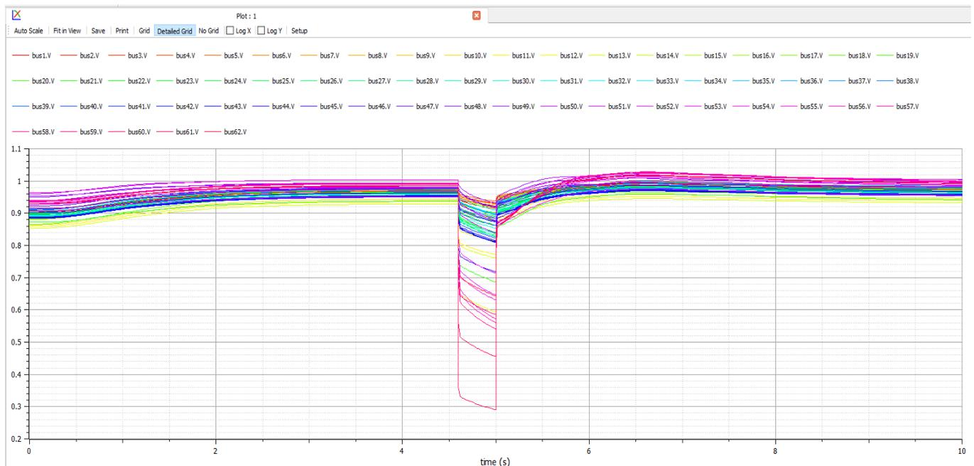
**Figure 3: The voltage profiles of simulated IEEE 62 bus.**
