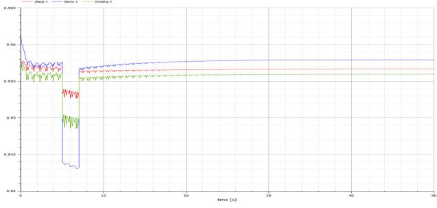
Figure 3: Voltage profiles of Alaoji Benin and Onitsha buses
