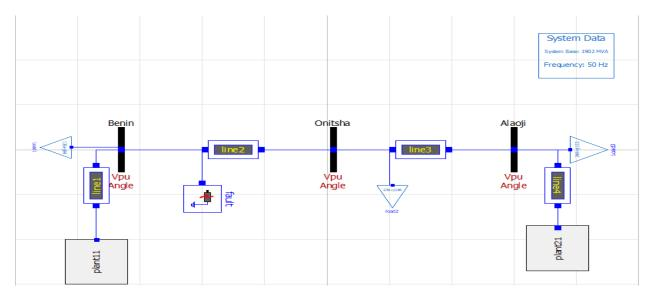
Figure 1: Modelling of Benin, Onitsha and Alaoji lines (330Kv) using Modelica and the OpenIPSL
