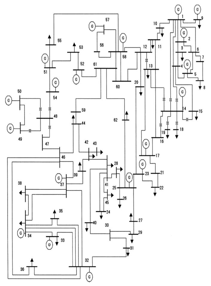
Figure 2: Single line diagram (SLD) of IEEE 62 bus system.
