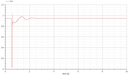
Figure 2: Voltage profile at the fault bus
