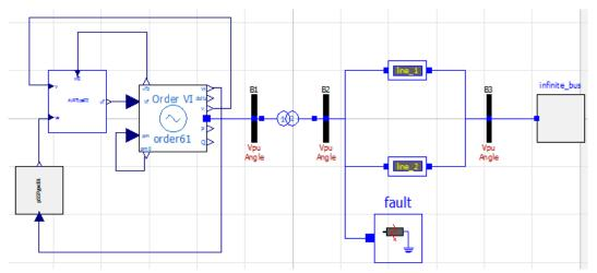
Figure 1: Implementation of SMIB using OpenIPSL
